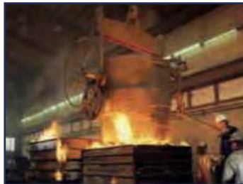
10.000 kg of metal being poured
