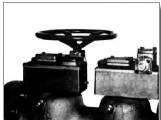
The gear has fixed stops at extreme position, plus position indicator
